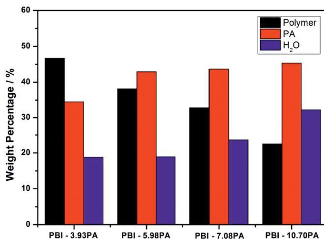
Fig. 17 Percentage composition of BTBP-PBI membranes treated by PA at different concentrations.
