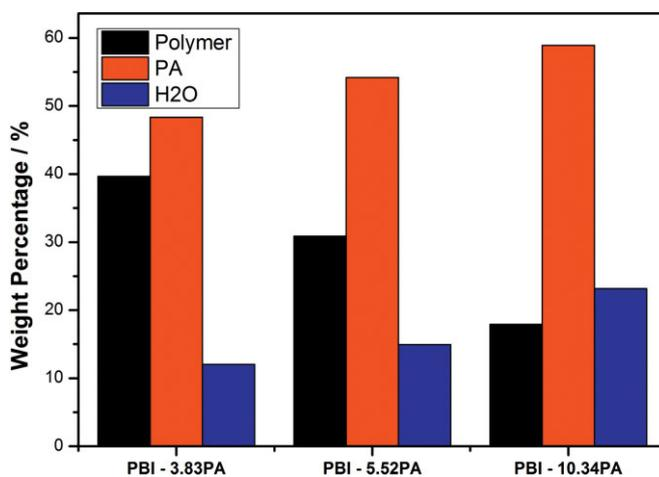
Fig. 18 Percentage composition of *meta*-PBI membranes treated by PA at different concentrations.
