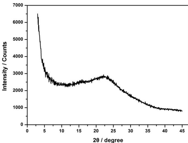
Fig. 13 WAXRD pattern of BTBP-PBI dense film.
