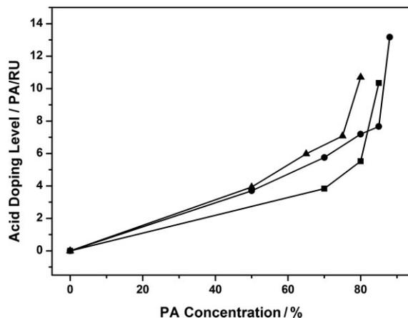
Fig. 14 PA doping levels of BTBP-PBI membranes (triangles), *meta*-PBI (squares) and 6F-PBI membranes (circles) treated by PA at different concentrations.
