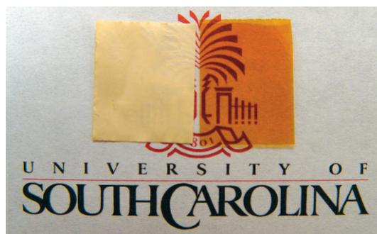
Fig. 12 BTBP-PBI dense films (left: dried under air; right: dried under nitrogen).
