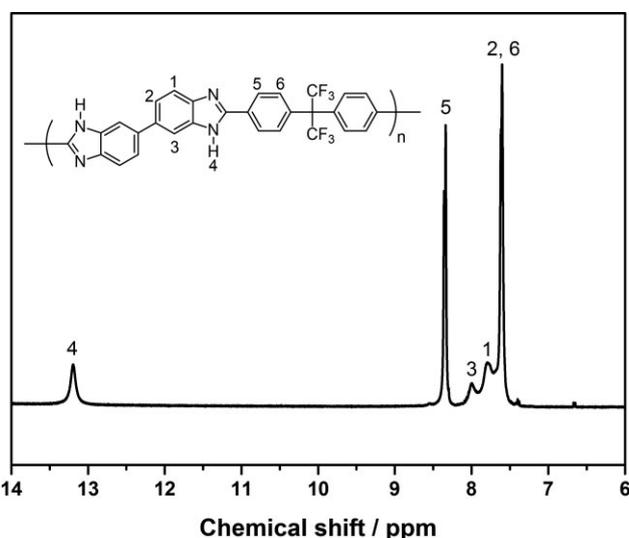
Fig. 8  $^1\text{H}$  NMR spectrum of 6F-PBI in  $\text{DMSO-d}_6$ .
