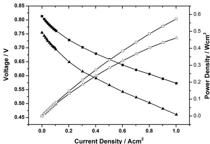
Fig. 21 Polarization curves (filled symbols) and power density curves (unfilled symbols) for MEA using BTBP-PBI membrane. (Fuel cell operation conditions: 1 atm, 180 °C, constant stoichiometry H<sub>2</sub> ( $\lambda = 1.2$ )/air ( $\lambda = 2.0$ ) (triangles) or ( $\lambda = 1.2$ )/O<sub>2</sub> ( $\lambda = 2.0$ ) (squares), no external humidification).
