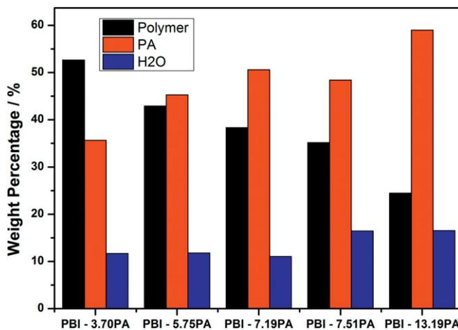
Fig. 19 Percentage composition of 6F-PBI membranes treated by PA at different concentrations.
