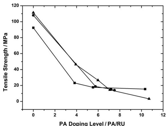
Fig. 15 Tensile Strength of PBI membranes (triangles: BTBP-PBI, squares: meta-PBI, circles: 6F-PBI) as a function of PA doping level at ambient temperature.
