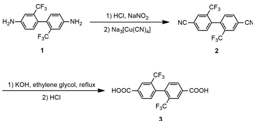
Fig. 1 Synthesis of 2,2'-bis(trifluoromethyl)-4,4'-biphenyldicarboxylic acid.
