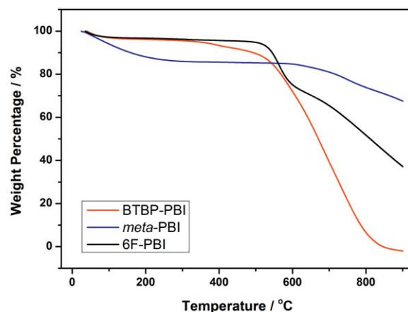
Fig. 11 TGA thermograms of BTBP-PBI, *meta*-PBI and 6F-PBI in nitrogen atmosphere.
