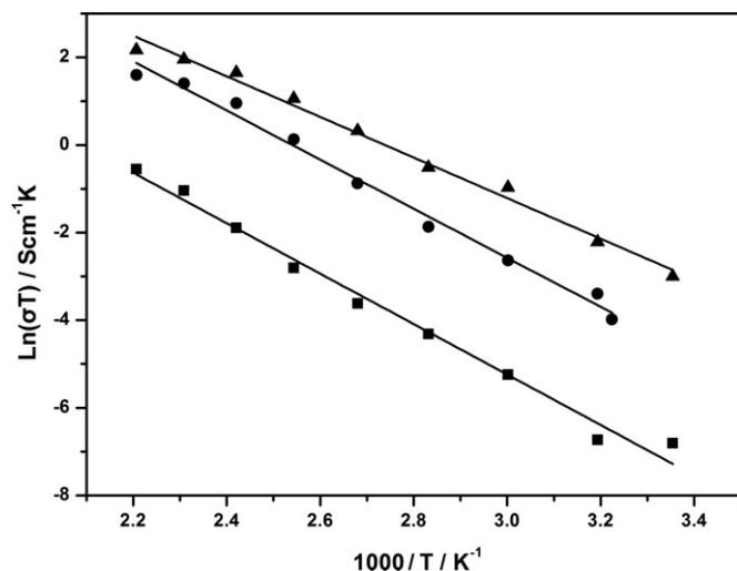
Fig. 20 Temperature dependence of proton conductivity of BTBP-PBI membranes without humidification. PA doping levels of PTBP-PBI membranes: (squares) 3.93 mole/RU; (circles) 5.98 mol/RU; (triangles) 7.08 mol/RU.
