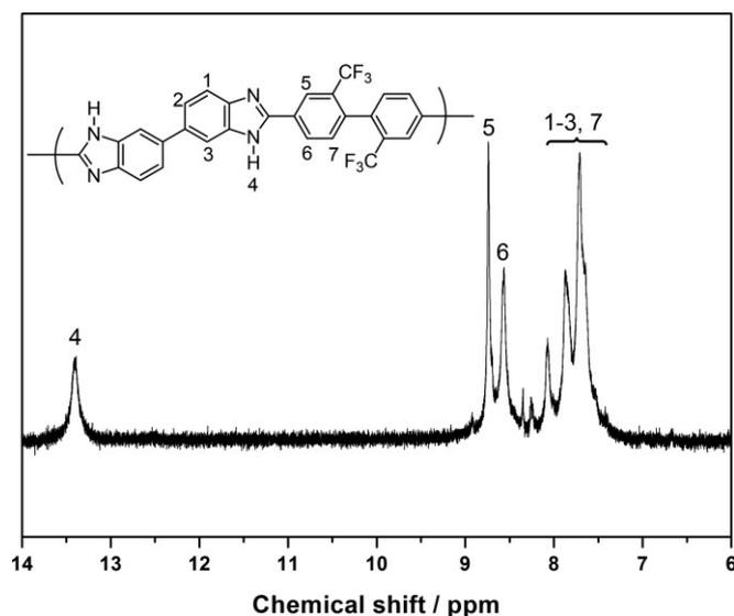
Fig. 6 <sup>1</sup>H NMR spectrum of BTBP-PBI in DMSO-d<sup>6</sup>.
