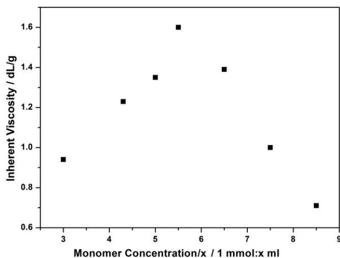
Fig. 3 Effect of monomer concentration on IV for BTBP-PBI at a polymerization temperature of 140 °C.
