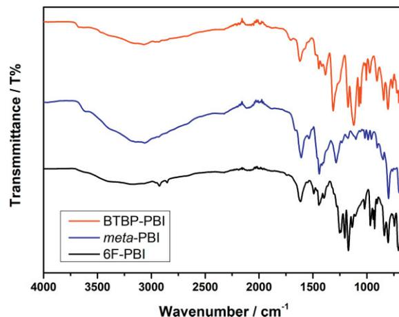
Fig. 5 FTIR spectra of BTBP-PBI, *meta*-PBI and 6F-PBI.
