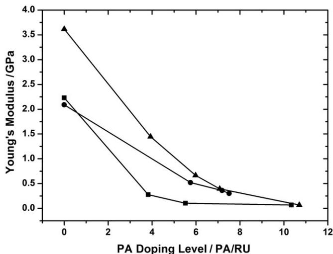
Fig. 16 Young's modulus of PBI membranes (triangles: BTBP-PBI, squares: meta-PBI, circles: 6F-PBI) as a function of PA doping level at ambient temperature.
