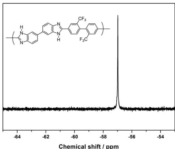
Fig. 9  $^{19}\text{F}$  NMR spectrum of BTBP-PBI in  $\text{DMSO-d}_6$ .
