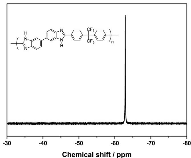
Fig. 10  $^{19}\text{F}$  NMR spectrum of 6F-PBI in  $\text{DMSO-d}_6$ .
