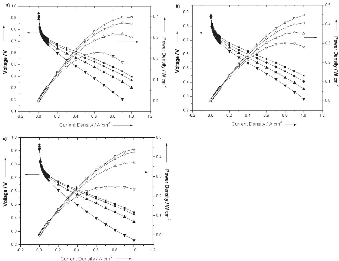
Fig. 5 Hydrogen–air fuel cell performance (180 °C, closed squares; 160 °C, closed circles; 140 °C, closed triangles; 120 °C, closed inverted triangles) and power density curves (180 °C, open squares; 160 °C, open circles; 140 °C, open triangles; 120 °C, open inverted triangles) for (a) 40/60 s-PBI/*p*-PBI segmented block copolymer, (b) 50/50 s-PBI/*p*-PBI segmented block copolymer and (c) 60/40 s-PBI/*p*-PBI segmented block copolymer.
