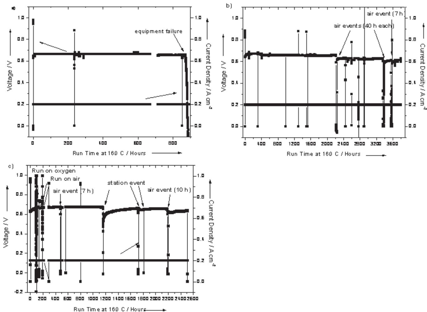
Fig. 6 Long-term hydrogen–air performance at 160 °C and 0.2 A cm<sup>-2</sup> for (a) 40/60 s-PBI/p-PBI segmented block copolymer, (b) 50/50 s-PBI/p-PBI segmented block copolymer and (c) 60/40 s-PBI/p-PBI segmented block copolymer.
