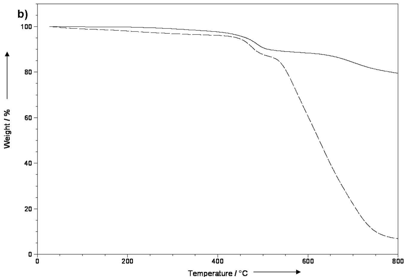
Fig. 1 (a) TGA in nitrogen of *p*-PBI and representative examples of segmented block copolymers (90/10 *s*-PBI/*p*-PBI, closed circles; 60/40 *s*-PBI/*p*-PBI, open circles; 40/60 *s*-PBI/*p*-PBI, open diamonds; *p*-PBI, closed diamonds) and relationship between *s*-PBI content and weight loss over 425–525 °C (inset); (b) TGA in nitrogen (solid line) and air (dashed line) of a representative block copolymer (50/50 *s*-PBI/*p*-PBI).
