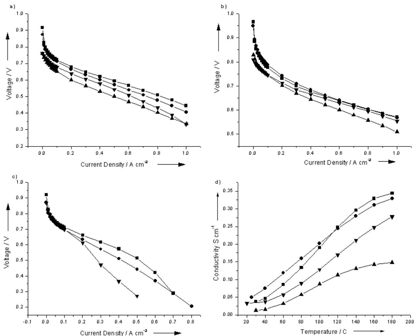
Fig. 10 Fuel cell performance and proton conductivity comparisons of the s-PBI (▼) and p-PBI (■) homopolymers with the 50/50 s-PBI/p-PBI random copolymer (▲) and 50/50 s-PBI/p-PBI block copolymer (●) for (a) hydrogen-air (160 °C); (b) hydrogen-oxygen (160 °C); (c) reformate-air (160 °C); and (d) proton conductivity at different temperatures.
