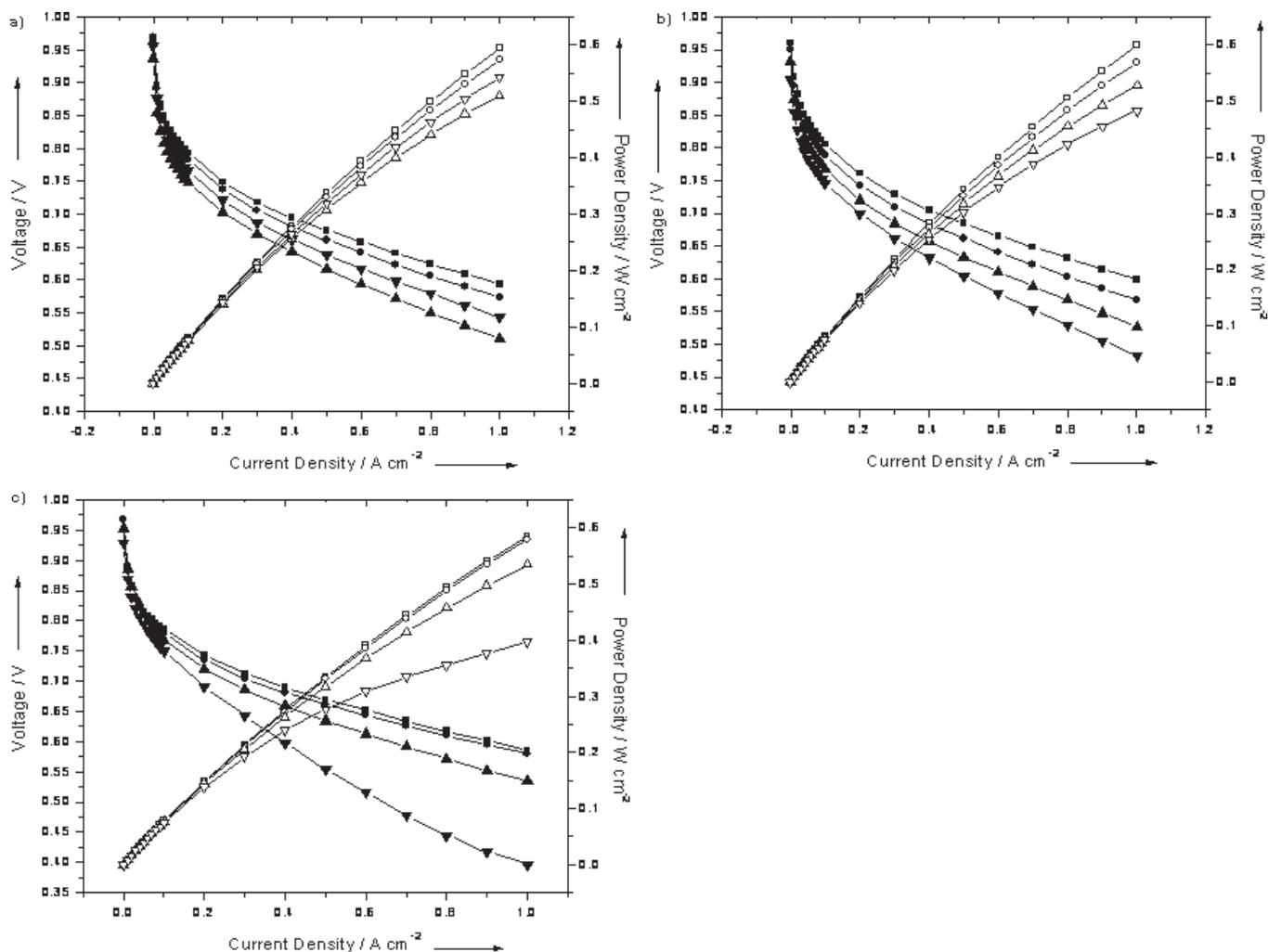
Fig. 7 Hydrogen–oxygen fuel cell performance (180 °C, closed squares; 160 °C, closed circles; 140 °C, closed triangles; 120 °C, closed inverted triangles) and power density curves (180 °C, open squares; 160 °C, open circles; 140 °C, open triangles; 120 °C, open inverted triangles) for (a) 40/60 s-PBI/*p*-PBI segmented block copolymer, (b) 50/50 s-PBI/*p*-PBI segmented block copolymer and (c) 60/40 s-PBI/*p*-PBI segmented block copolymer.
