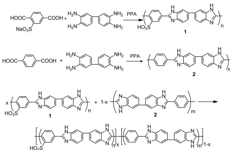
Scheme 1 Synthesis of *s*-PBI/*p*-PBI segmented block copolymers.
