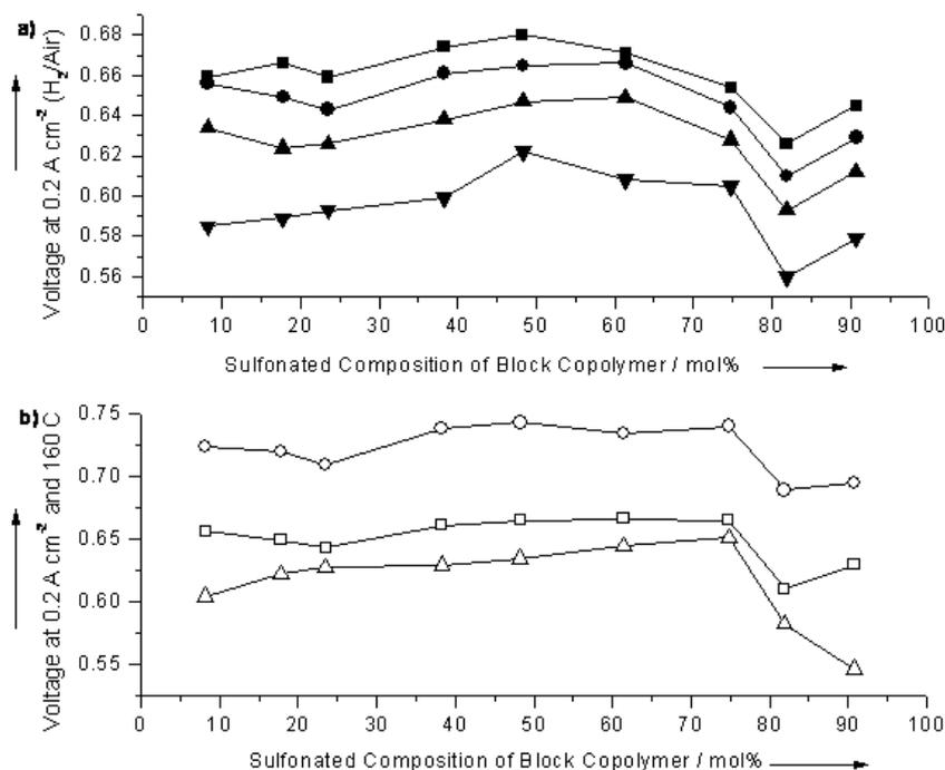
Fig. 4 s-PBI/p-PBI segmented block copolymer fuel cell performance with (a) hydrogen–air at different temperatures (180 °C, squares; 160 °C, circles; 140 °C, triangle; 120 °C, inverted triangle) and (b) different fuels and oxidants at 160 °C (H<sub>2</sub>-Air, open squares; H<sub>2</sub>-O<sub>2</sub>, open circles; Reformat-Air, open triangles).
