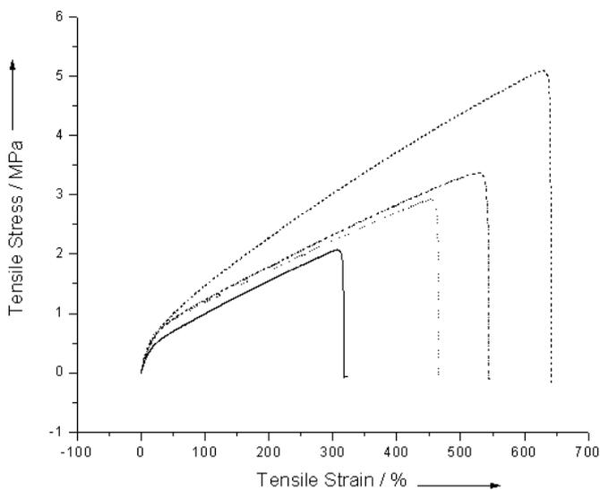
Fig. 3 Tensile stress–strain curves of 10/90 s-PBI/*p*-PBI segmented block copolymer (dashed line, ---), 25/75 s-PBI/*p*-PBI segmented block copolymer (dash-dot line, -.-), 20/80 s-PBI/*p*-PBI segmented block copolymer (dotted line, .....), 50/50 s-PBI/*p*-PBI segmented block copolymer (solid line, -).
