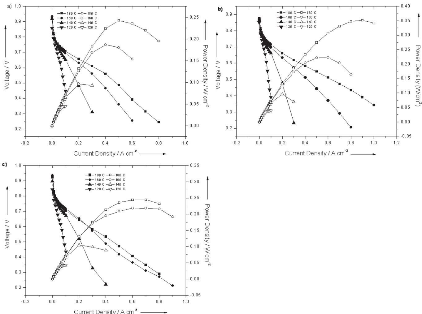
Fig. 8 Reformate-air fuel cell performance (180 °C, closed squares; 160 °C, closed circles; 140 °C, closed triangles; 120 °C, closed inverted triangles) and power density curves (180 °C, open squares; 160 °C, open circles; 140 °C, open triangles; 120 °C, open inverted triangles) for (a) 40/60 s-PBI/*p*-PBI segmented block copolymer, (b) 50/50 s-PBI/*p*-PBI segmented block copolymer and (c) 60/40 s-PBI/*p*-PBI segmented block copolymer.
