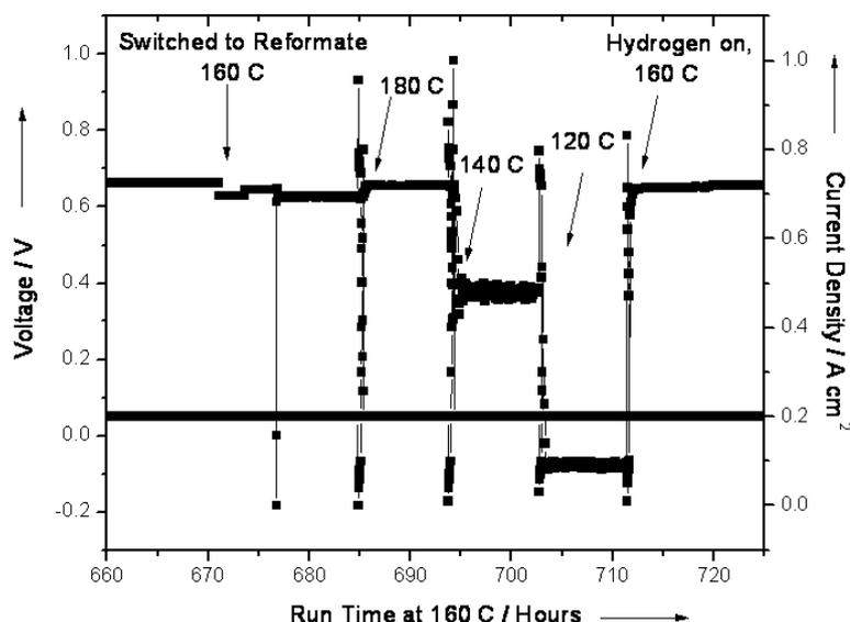
Fig. 9 Reformat recovery study of the 40/60 s-PBI/p-PBI segmented block copolymer. The cell was run for 8 h at each temperature with reformat gas, then hydrogen gas was used as the fuel at 160 °C.
